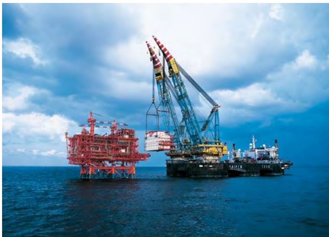
Figure 14: Conventional HLV, in this case Saipem 7000, lifting a topsides structure
